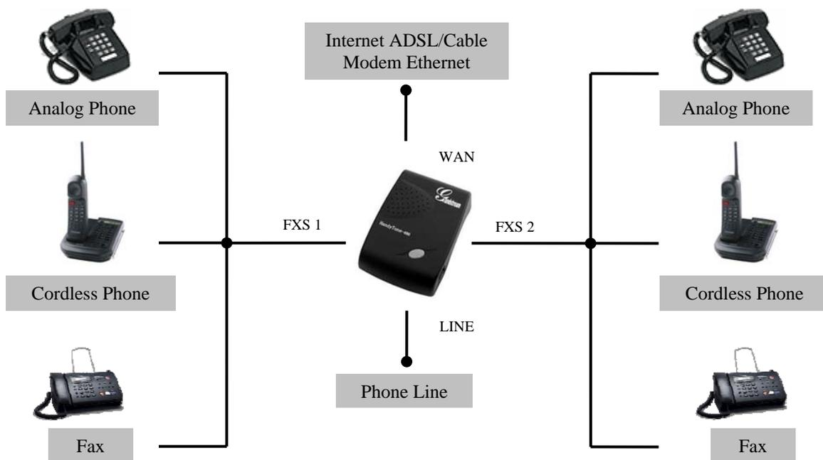
HandyTone-386 has two FXS ports. The RJ11 jack next to the WAN is called FXS port 2 and the RJ11 jack on the corner is called FXS port 1. The RJ11 jack on the side on of the HandyTone-386 is a LINE port. Each FXS port can have a separate SIP account. This is a key feature of HandyTone-386. Both ports can make calls concurrently.
